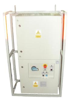
Switchgear type KTON-05W/2(4,X) is an electric an device designed for use underground mining, in workpits in non-explosive hazard conditions and on the ground in non-hazardous areas.
